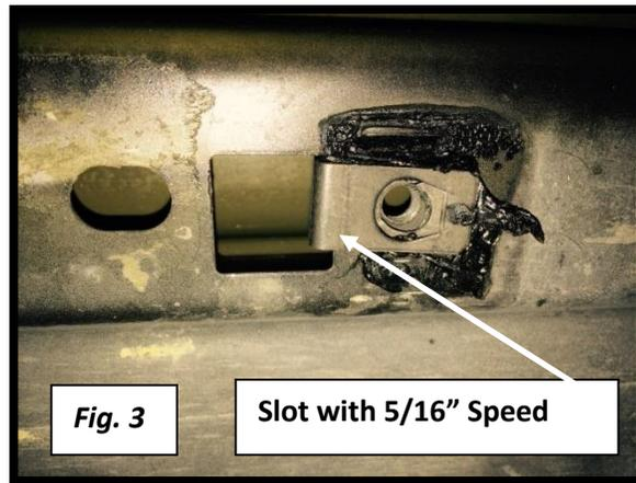
**Step. 4** Starting with the passenger side, carefully raise bar up to the pinch weld of the body and align the pinch weld tabs with the Factory mounting holes. Loosely install the 5/16" Hex bolts, washers & nuts. Do NOT fasten down tightly, as you may need to lightly adjust the bar upon applying remaining locations. **Note: Some models may require the drilling out of additional 5/16 mounting holes in each pinch weld tab location.**
