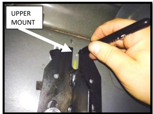
**Step 5:** Remove Nerf Step and set aside. Next, slide the additional 3/8 threaded clip from the upper rectangle hole and align with the “U” shaped mark from step 5. Make a mark through the threaded part of the clip.
