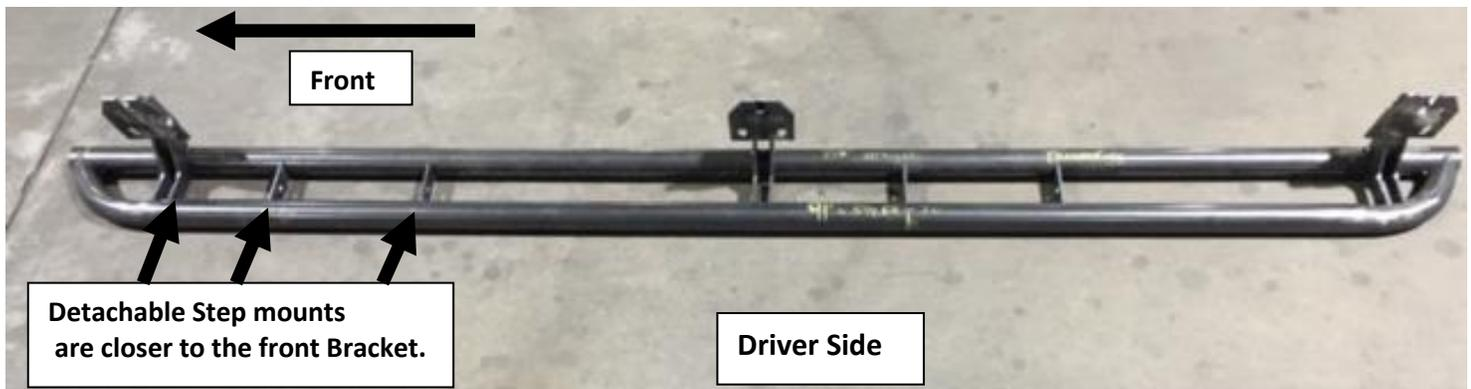
**Step 3:** Using the 3/8" threaded clips, slide two clips in the upper rectangular hole, and align one clip in each hex hole so the clip threads are visible. **Figure 1**
