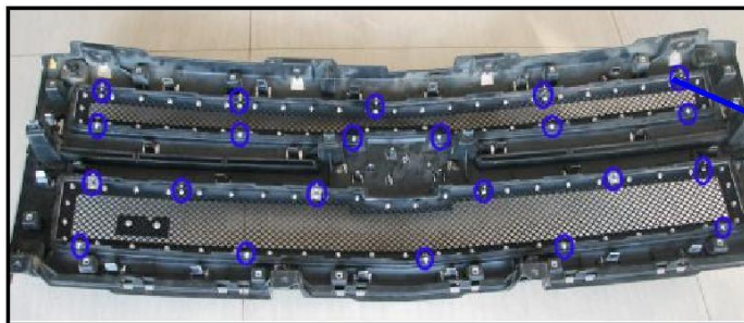
Figure 3 – Rear view of vehicle's shell; Grills attached with Metal Brackets and Flange Nuts
