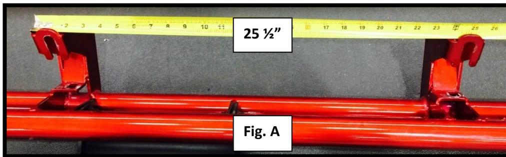
**Step 2:** With the correct rail is placed on each side of the vehicle, take note of where the brackets are located. Look on the underside of the body and locate the factory supplied mounting positions. **NOTE:** Some vehicles require the use of speed clips and nuts which are supplied with the hardware kit.
